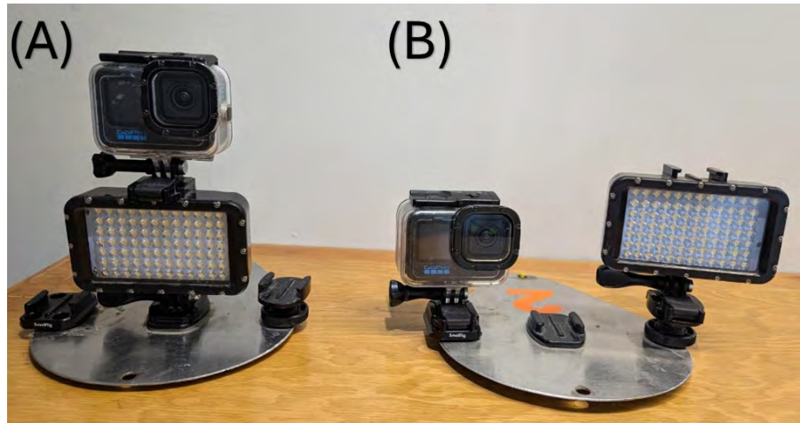
Figure 3: GoPro HERO 12 Cameras with stainless steel mount and Suptig 84-LED lights. Different camera mount set ups denoted A and B depending on requirements.
