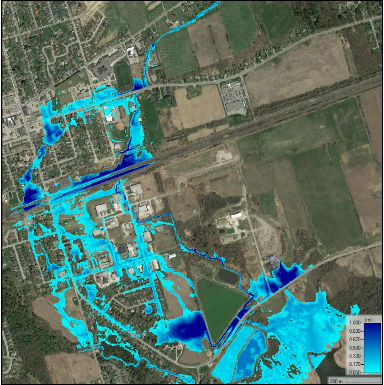
Figure 8-7: Draft Inundation Boundary for Arena Creek in Timmins Storm
