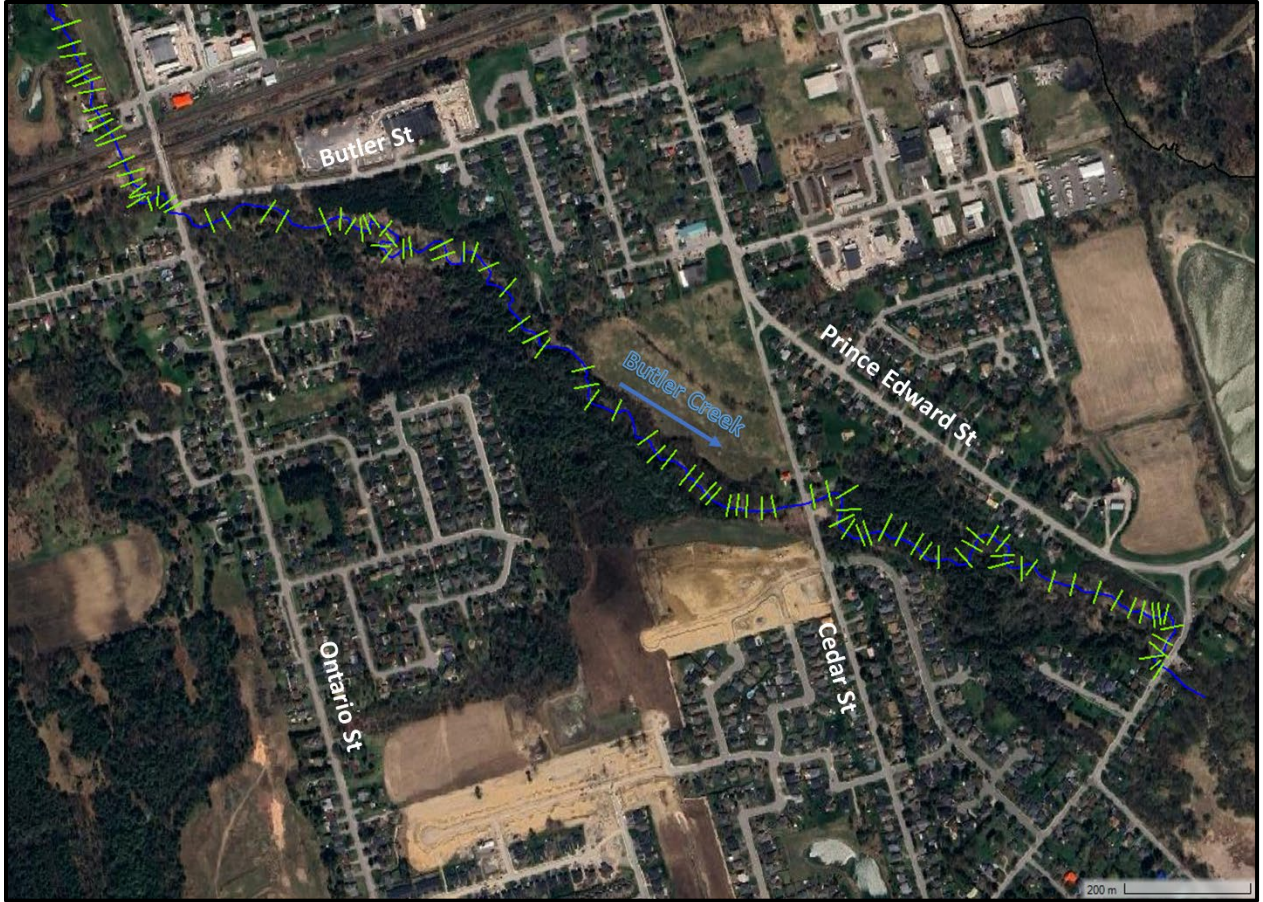
Figure 5-2: Locations of Surveyed Bathymetry Sections within Butler Creek Study Area Downstream of Ontario St
