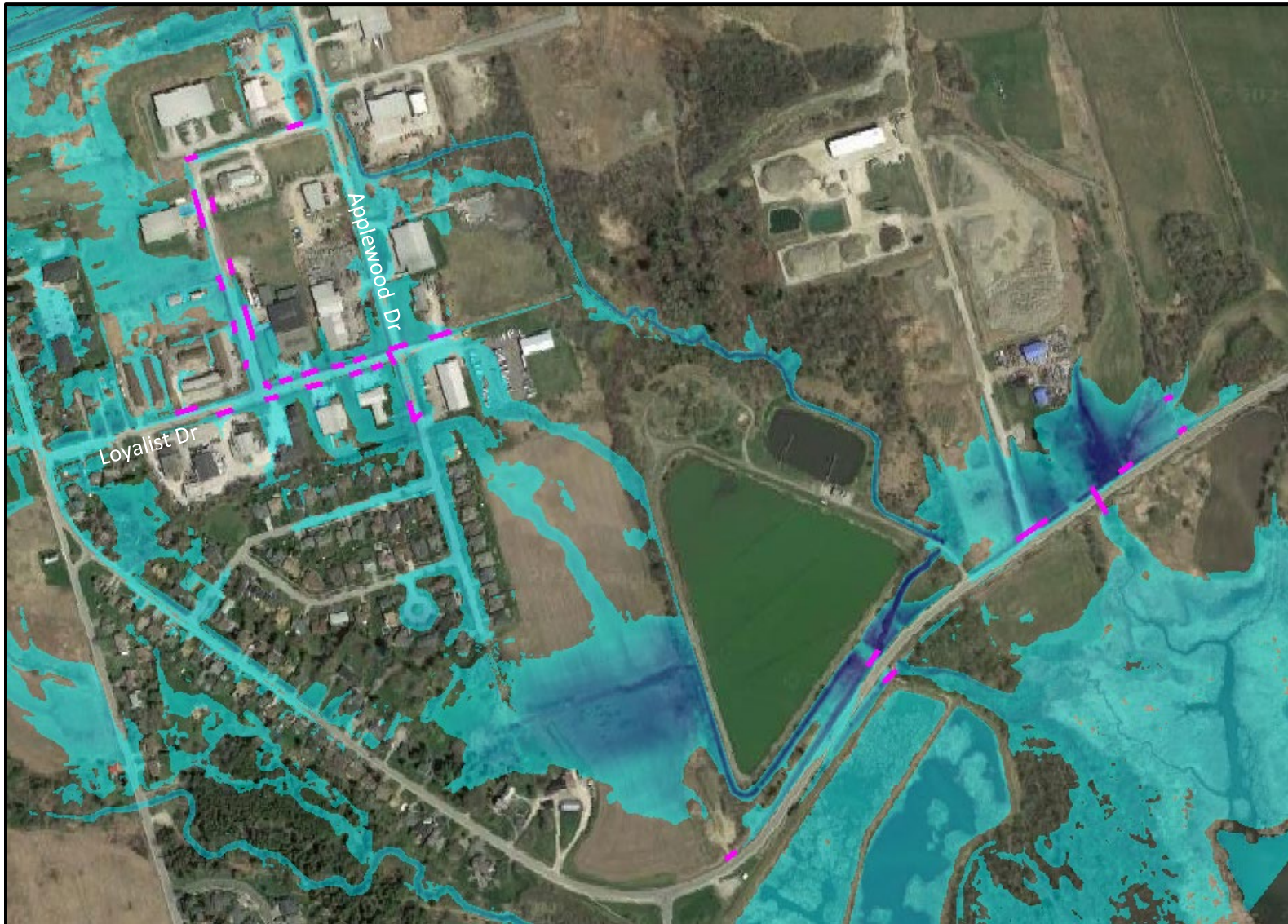
Figure 8-4: Location of Connection Culverts Included in HEC-RAS Model; Timmins Depth Layer Overlay
