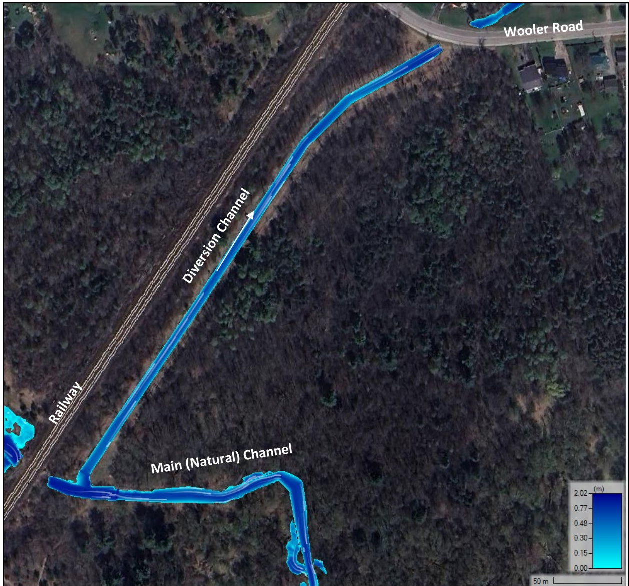
Figure 5-37: Mayhew Creek Natural Channel and Constructed Diversion Channel Downstream of Railway Tracks
