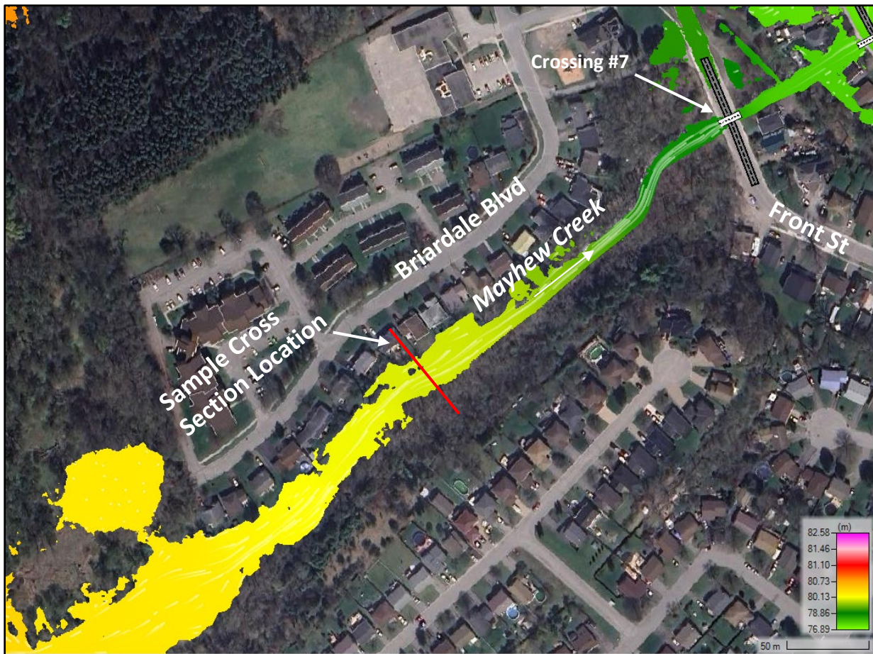
Figure 5-20: Schematic of Timmins Floodplain Upstream of Crossing #7; Timmins Water Level Overlay
