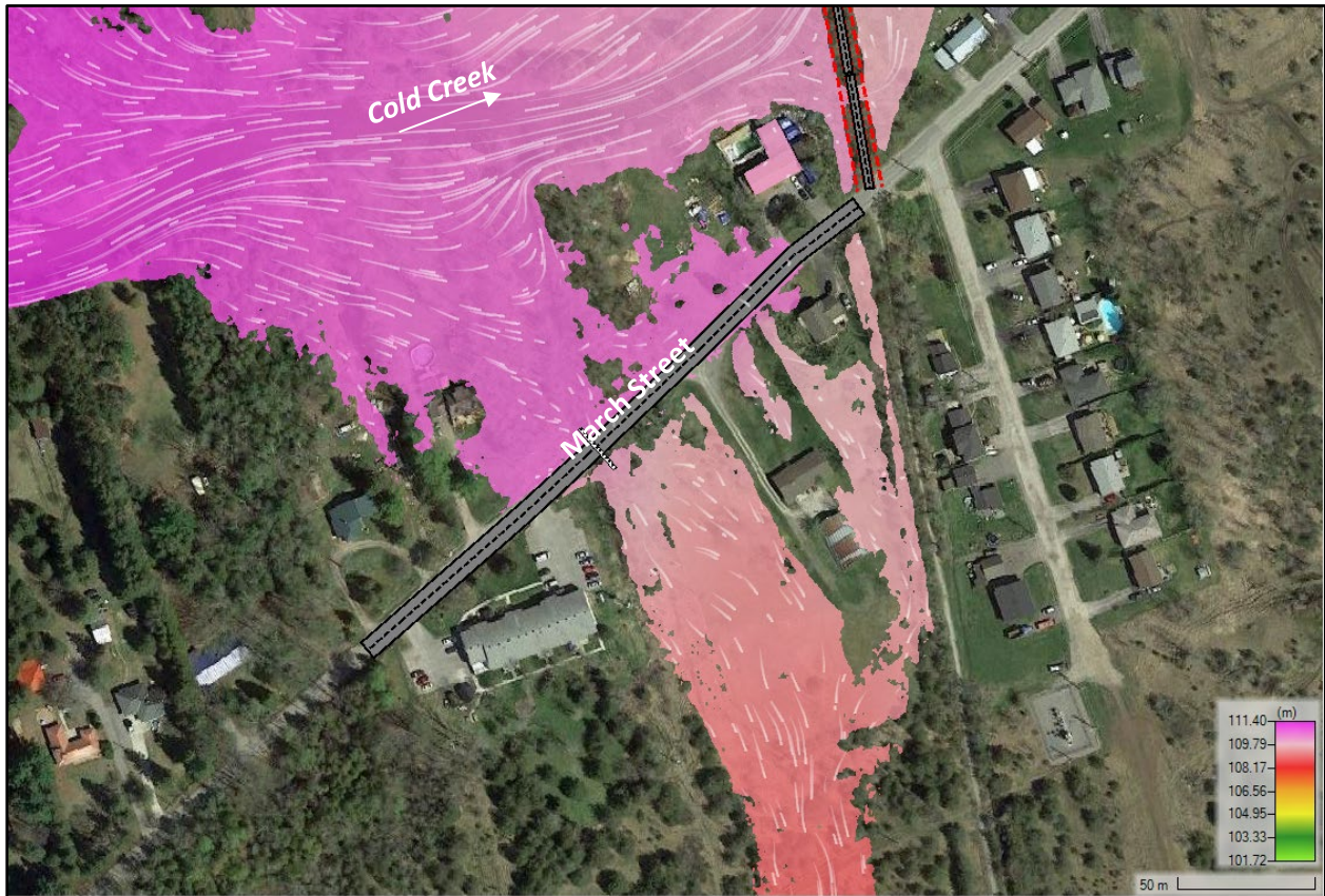
Figure 6-12: Timmins Inundation Area in Vicinity of March Street Spill Crossing; Water Level Overlay
