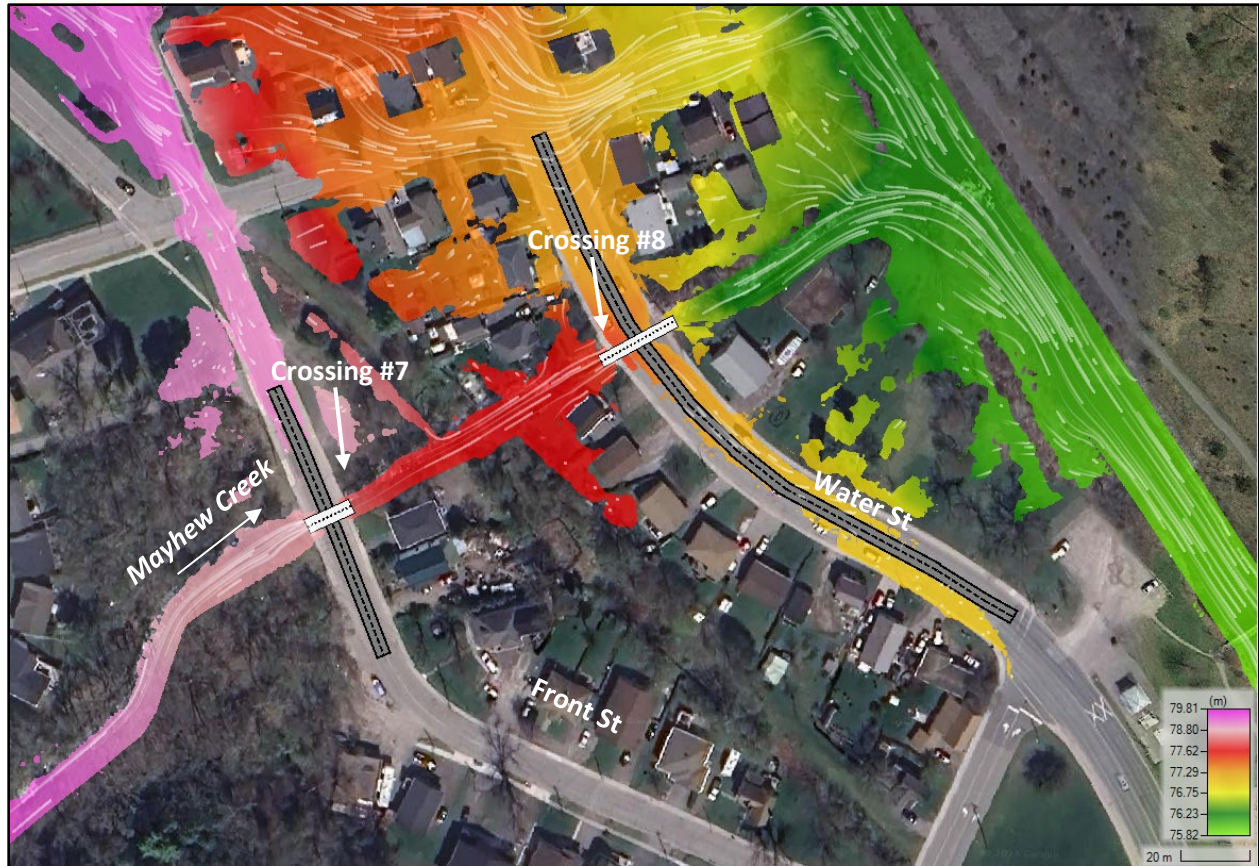
Figure 5-23: Timmins Inundation Boundary in Vicinity of Crossings #7 and 8
