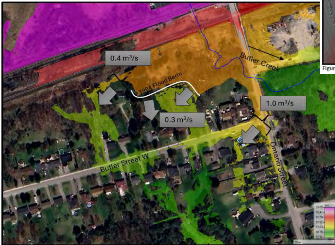
Figure 5-26: Ontario Street Spill Towards Butler Street West; Timmins WSEL Overlay
