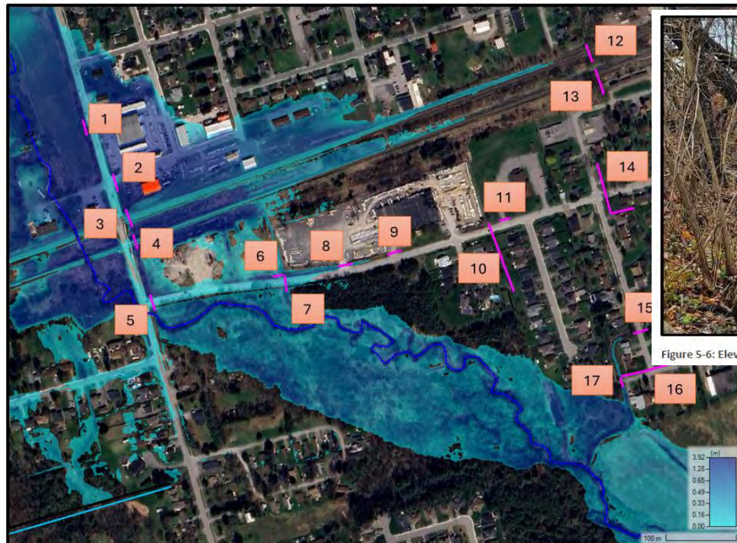
Figure 5-5: Connection Culvert Locations Included for Navigating Butler Creek Spill Near Ontario Street and Butler Street
