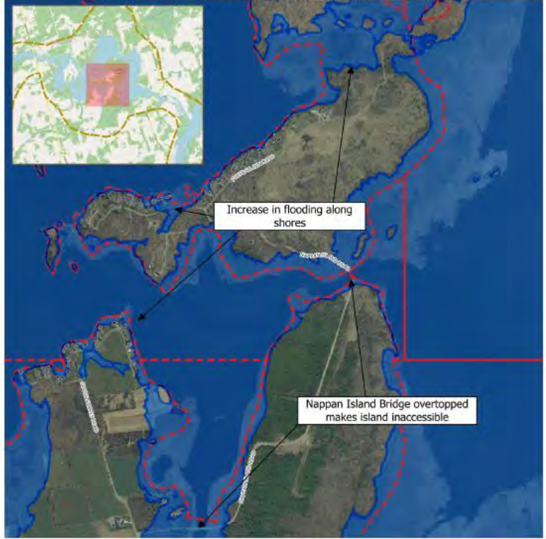
FIGURE 3-21: FLOODLINES AT NAPPAN ISLAND
