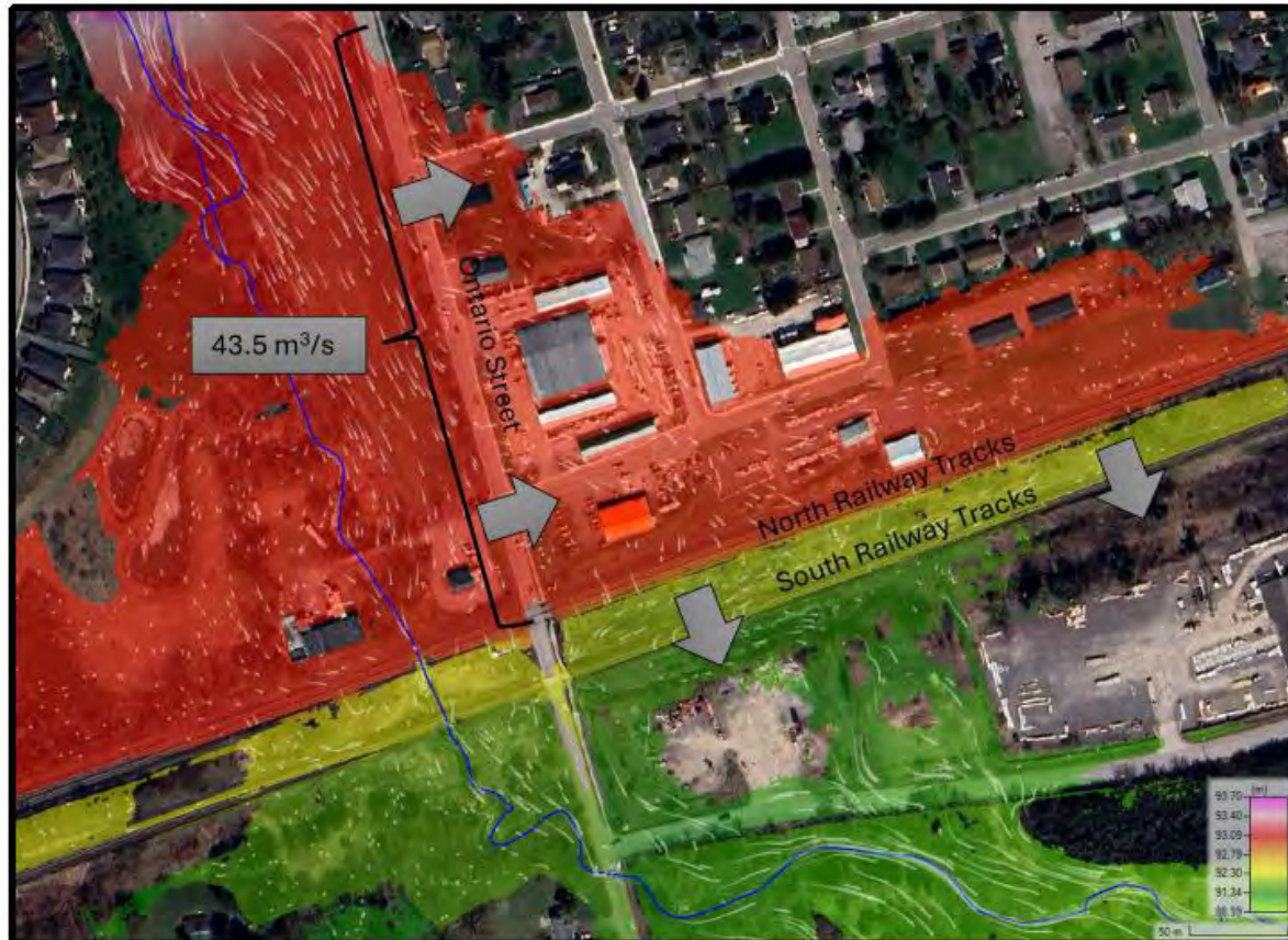
Figure 5-24: Spill East of Ontario Street, North of Railway Tracks; Timmins WSEL Overlay
