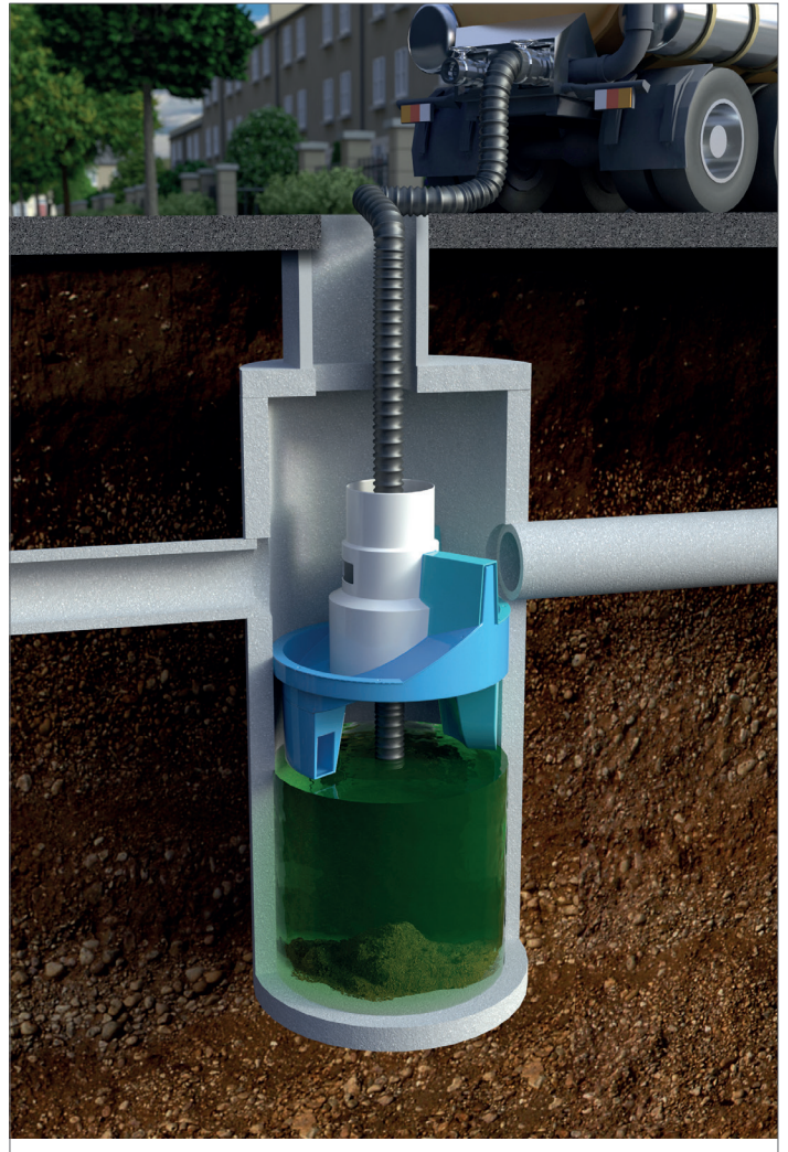
Fig.4 Floatables are removed with a vactor hose
