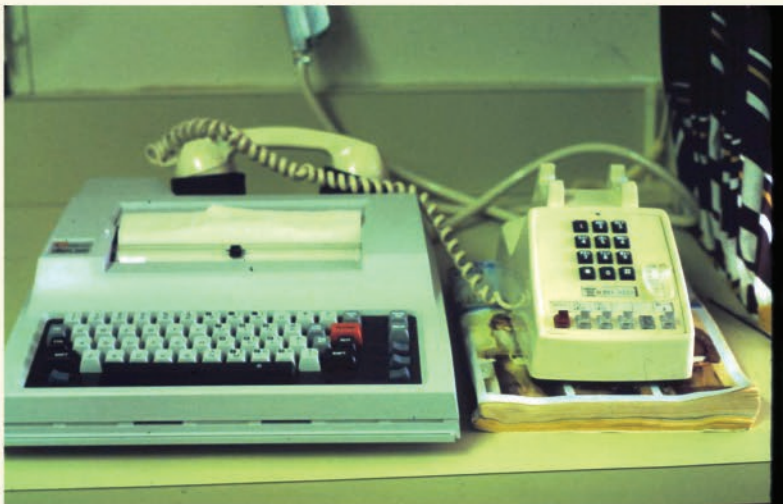
ENVOY 100 used a telephone line and modem to remotely communicate monitoring data
